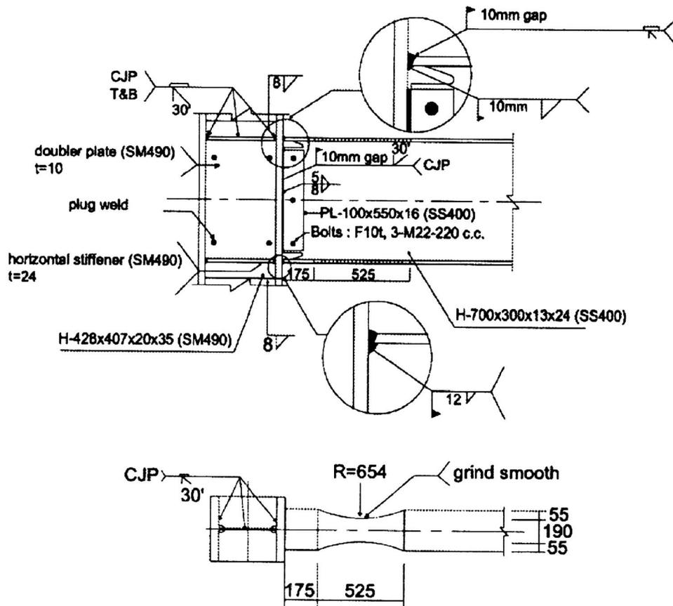
Fig. 3. Specimen *DB700-SW* moment connection details
