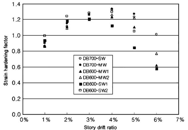
**Fig. 16.** Story drift ratio versus strain hardening factor in welded-web specimens
