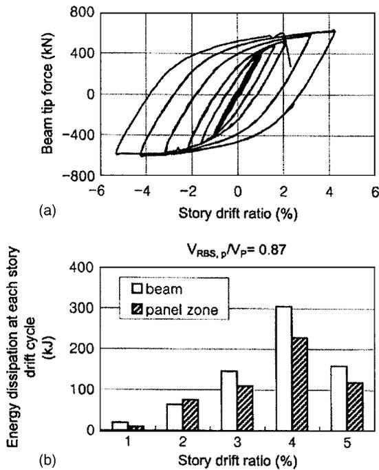
**Fig. 17.** Global response and energy dissipation (specimen *DB700-MW*): (a) global response and (b) energy dissipation at each story drift cycle
