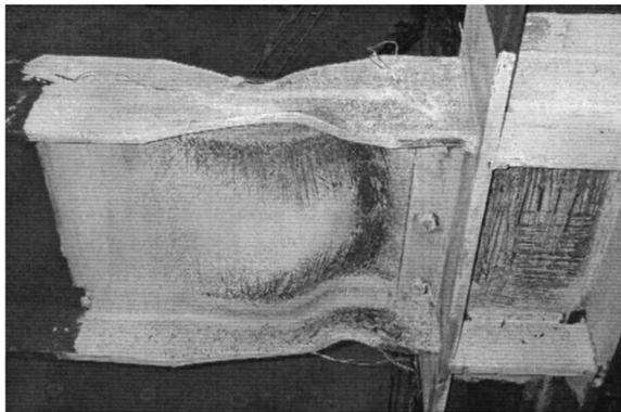
Fig. 9. Connection region of specimen *DB700-SW* at 6% story drift
