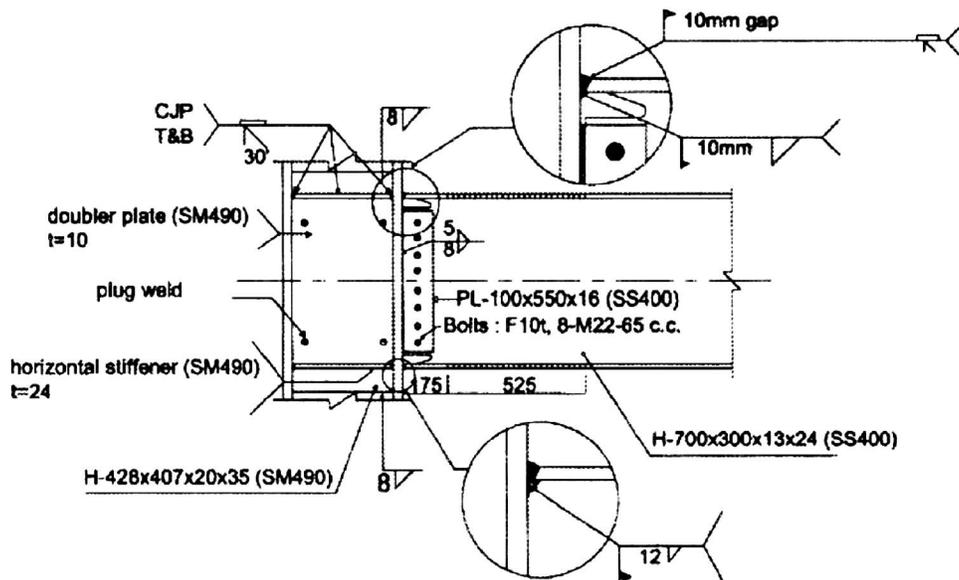
Fig. 4. Specimen *DB700-SB* moment connection details
