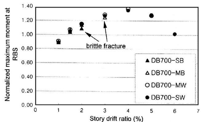
Fig. 12. Comparison of normalized maximum moment at reduced beam section (Set number 1)
