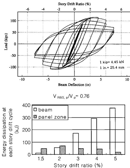
**Fig. 18.** Global response and energy dissipation at each story drift cycle (specimen *LSI*)
