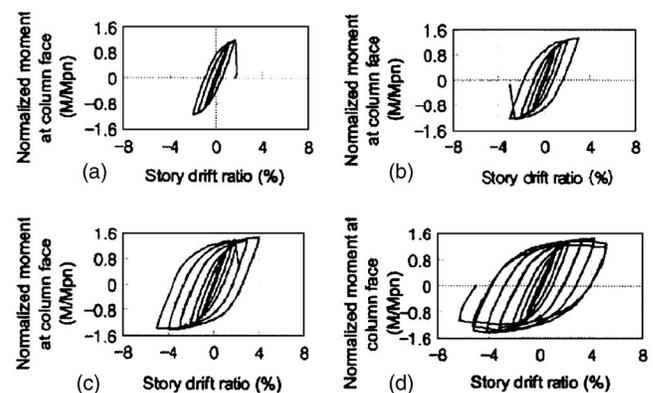
Fig. 7. Normalized moment versus story drift ratio relationship (set number 1): (a) *DB700-SB*, (b) *DB700-MB*, (c) *DB700-MW*, and (d) *DB700-SW*
