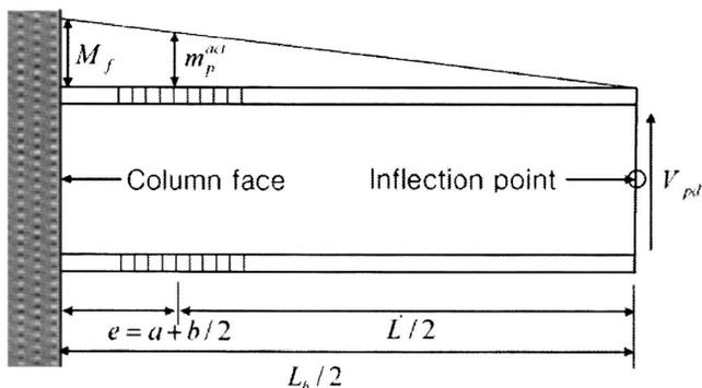
Fig. 2. Seismic moment profile for reduced beam section design
