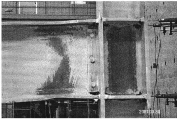
Fig. 8. Connection region of specimen *DB700-MW* at 5% story drift
