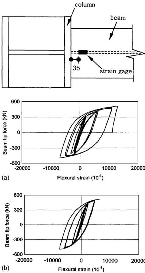
**Fig. 13.** Comparison of measured flexural strain responses near groove weld of beam bottom flange: (a) *DB700-SB* and (b) *DB700-SW*
