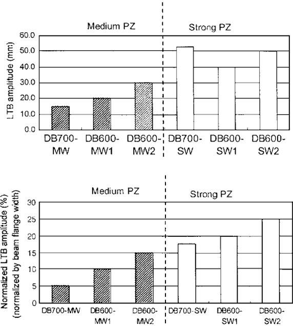
**Fig. 15.** Comparison of lateral-torsional buckling amplitudes at 4% story drift cycle: (a) absolute amplitude and (b) relative amplitude
