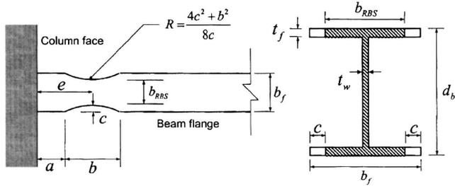
Fig. 1. Typical geometry of radius-cut reduced beam section
