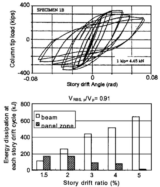
**Fig. 19.** Global response and energy dissipation at each story drift cycle (specimen *IB*)
