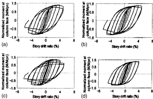
**Fig. 14.** Normalized moment versus story drift ratio relationship (set number 2): (a) *DB600-MW1*, (b) *DB600-MW2*, (c) *DB600-SW1*, and (d) *DB600-SW2*
