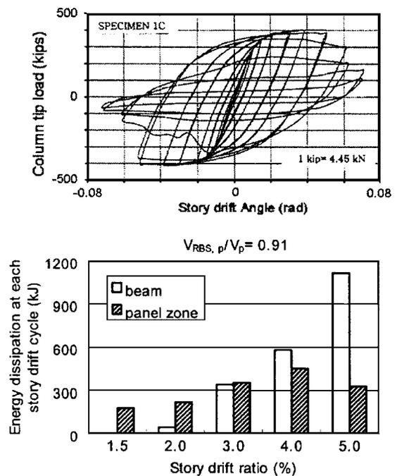
**Fig. 20.** Global response and energy dissipation at each story drift cycle (specimen *IC*)
